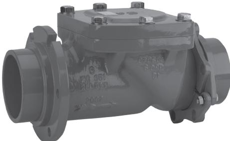
◀ **SA-Series Check Valve** – with integral 6” male mechanical joint ends to connect directly to any standard 6” MJ hydrant shoe connection without additional pipe. Convenient means to add protection with a minimum of additional joints. Similar to 250/HS check valve function and features.
