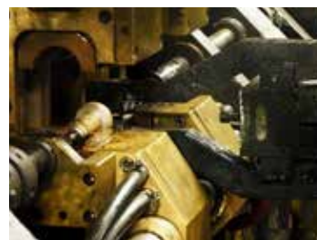
Stem is electrically heated and thrust together to create the thrust collar
