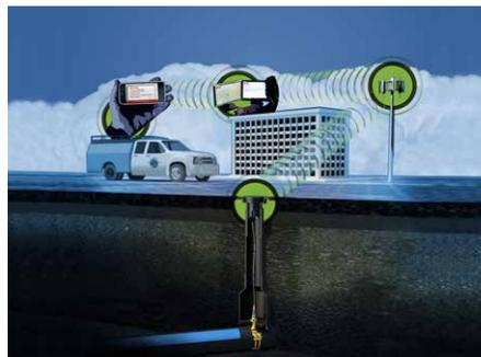
Mueller Co. has developed a simple and cost-effective technology to continuously monitor pressure in potable water distribution systems. This new remote pressure sensor system, typically installed two per District Metering Area (DMA) or pressure zone, reports at user-defined intervals via cellular service and a Mueller-hosted secure web server. Real-time alerts are sent when settings
