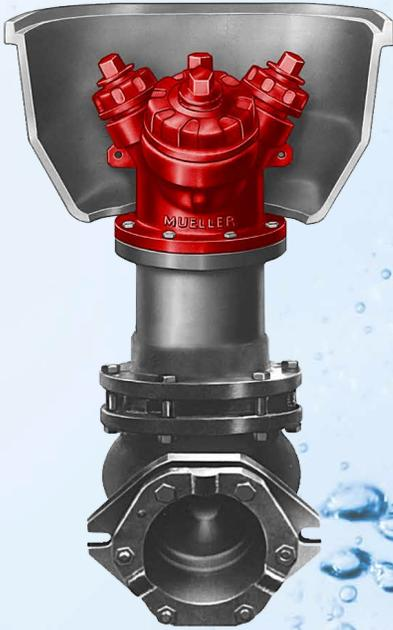
Mueller has re-designed the A-415 flush-type fire hydrant head assembly. By modifying the hold down nut, adding a thrust washer and implementing manufacturing process improvements, operating torque was significantly reduced. According to Product Manager Alan Channell, "These product improvements reduced operating torque by as much as 25% in field tests, which is especially helpful in higher pressure systems".
