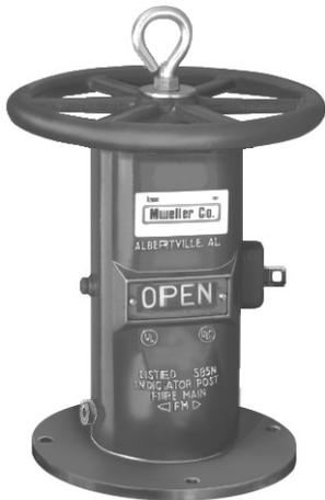
The Mueller Wall Mount Indicator Post is used to operate a valve installed behind a wall and indicates if that valve is open or shut. The Post has a 12" diameter base with 3/4" bolt holes which can be mounted to a wall.
