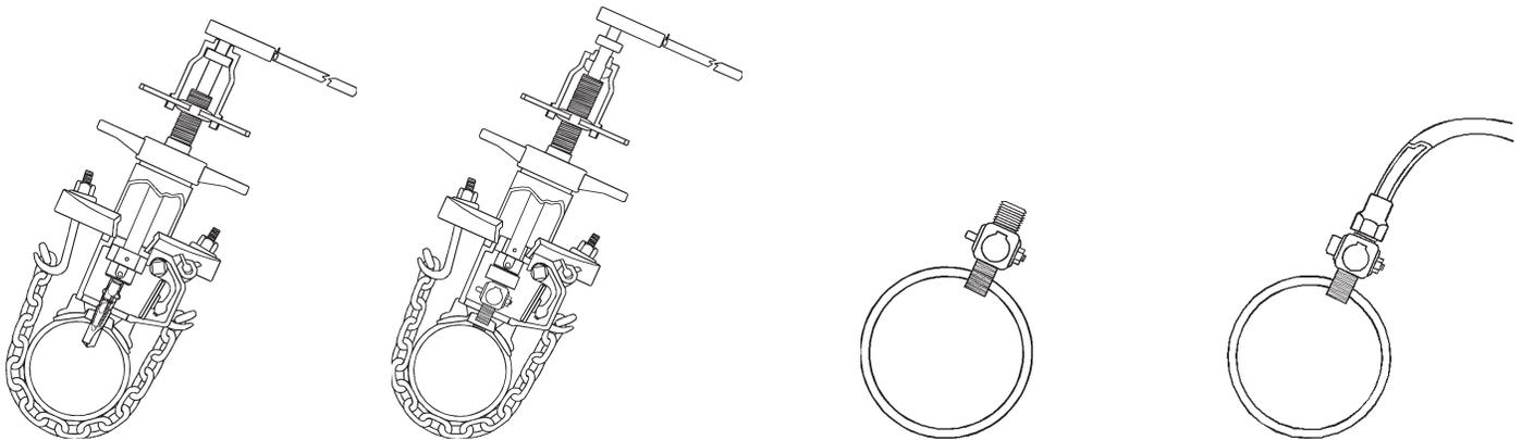
❑ MUELLER drilling and tapping machine drills and taps a hole in a pressurized main without allowing water to escape.
