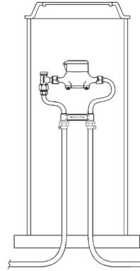
Typical installation of a vertical inlet and outlet copper meter yoke
