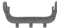
Iron meter yoke for 3/4" meters With stabilizing prongs to support yoke on 3/4" iron pipe stakes when yoke is attached to plastic service lines.
