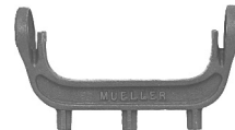
Iron meter yoke for 5/8" meters With stabilizing prongs to support yoke on 3/4" iron pipe stakes when yoke is attached to plastic service lines.
