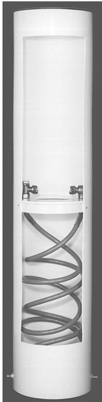
The MUELLER / Hunt THERMAL-COIL Meter Box provides a means to allow a meter to be read and maintained even though it is set deep in the ground to resist freezing. The THERMAL-COIL Meter Box is designed with the meter installed on a platform that normally sets near the bottom of the box where the ground temperature keeps it warmer. The meter and platform are connected to the service line by coils of polybutylene tubing which allow the meter and platform to be raised to the surface.
