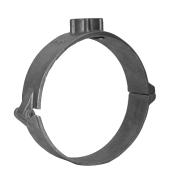
hinged saddles prevent deformation of the PVC that can be caused by over tightening a saddle with traditional straps, particularly if installed on non-pressurized pipe.
