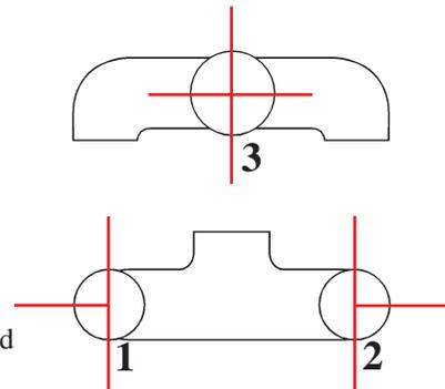
There are three possible locations where a special fitting can be attached: at outlets 1 and 2, or inlet 3.
