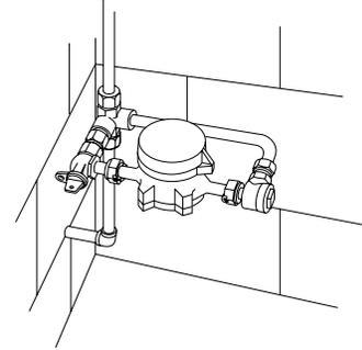
Typical installation of a horizontal inlet and outlet corner type copper meter yoke
