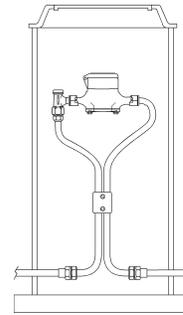
Typical installation of a flexible relocator
