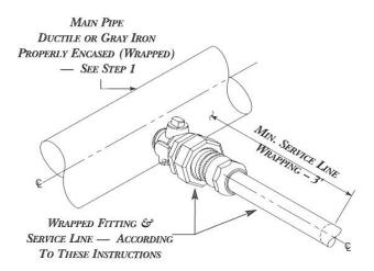
**CAUTION:** Read and follow these instructions to install the Mueller® Insulated Corporation Ball Valve. Failure to follow these instructions may result in damage to the valve and/or piping system, or may prevent the insulator from functioning as intended.
