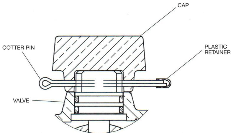
1. To install valve, remove cotter pin and cap from valve.
