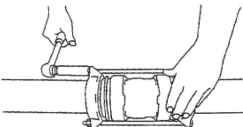
4. Slide the pipes into the AquaGrip coupling up to the marks made in step 3.
