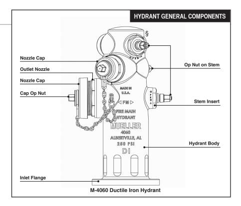
C600, "Standard for Installation of Ductile-Iron Water Mains and Their Appurtenances", and local fire codes for fire authority requirements. Always ensure an isolation valve is located between the hydrant and the main to permit the water supply to be cut-off for maintenance.
