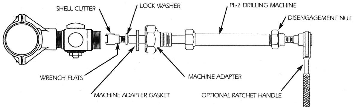
4. Lightly lubricate outside of shell cutter and boring bar of PL-2 machine BEFORE EACH USE. Use Mueller® Cutting Grease (part no. 88366) on cutter, and light machine oil (such as 3-1 brand oil) on boring bar.
