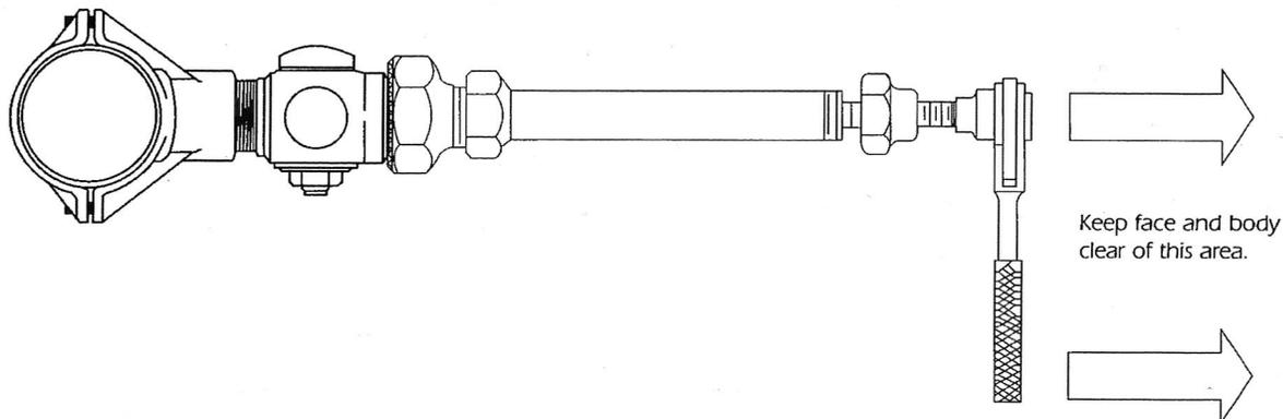
9. Remove machine and adapter from corporation valve as a unit. Do not insert any tool through slot in shell cutter to pry out the coupon – doing so could deform the cutter. Optional coupon removal tools (catalog no. 681242) will facilitate removal of coupon from shell cutter.
