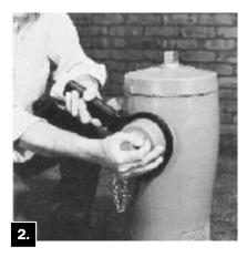
Place Nozzle Wrench behind threaded section of Nozzle so that Wrench gaps engage Nozzle drive lugs. Replace Nozzle Cap and tighten until Cap rests loosely against Wrench.
