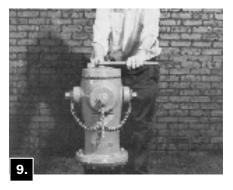
Unscrew one Hose Nozzle Cap slightly to bleed air. Open Hydrant fully. Tighten the Hose Nozzle Cap when water starts flowing and check all gaskets for leaks. Turn Operating Nut to fully CLOSED position and remove Hose Nozzle Cap to allow Barrel to drain. Replace Hose Nozzle Cap.
