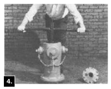
Straighten Stainless Steel Lock Washer, unscrew Cap Nut and remove Washer, Stem Seal, Lower Valve Plate, Main Valve and Seat Ring. Clean, inspect and replace any damaged parts. (On hydrants 1997 and newer, Main Valve can be reversed to provide new seal.) Replace Drain Valve Facings.Inspect and lubricate Top and Bottom Seat O-rings (replace if necessary). Lubricate all threaded surfaces and reassemble.
