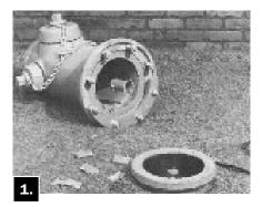
Mueller Hydrant with Upper Barrel knocked over by vehicle.
