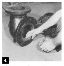
Lubricate new Shoe and Bottom Seat Ring O-ring.
