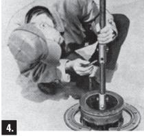
Assemble Upper Stem and Stem Coupling onto Extension Stem and retain it with stainless steel Clevis Pin and stainless steel Cotter Pin. Make sure Stem Coupling is installed with notches towards the Lower Stem, words "THIS END UP" towards the Upper Stem.
