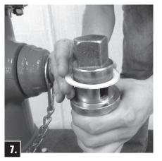
Check Bonnet O-ring\* for proper position and condition. Attach Brass Sleeve to Upper Stem and lubricate outside to protect O-ring Seals from thread damage. Place Bonnet onto Upper Barrel and assemble Bonnet Bolts only hand-tight. Remove Brass Sleeve. Reassemble Operating Nut, Anti-Friction Washer, and Hold-Down Nut (snug-tighten). Be sure O-ring Seals are in good condition at thread shoulder on outside of Hold-Down Nut and on inside where contact is made with Operating Nut.
