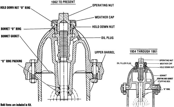
NOTE: Brass Sleeve A-366 will be required to remove the Bonnet in order to replace the two Packing "O" Rings (H-93).
