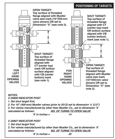
**11.** Using the Wrench, open and close the valve and check to see that the "SHUT" and "OPEN" Targets are clearly in view in the Windows, at their respective positions, and that there is no feeling of binding of the Upper or Lower Stem Assemblies. It is recommended that the turns to open/close be counted and compared to the valve manufacturer's specification, in order to verify full valve opening.
