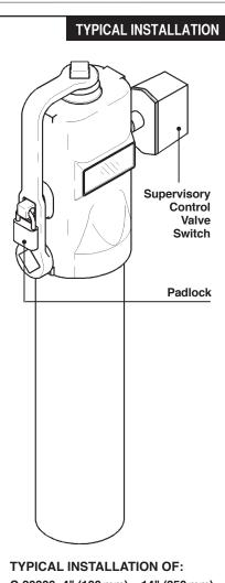
C-20806: 4" (100 mm) – 14" (350 mm) Post Indicator Valves C-20807: 16" (400 mm) – 24" (600 mm) Post Indicator Valves
