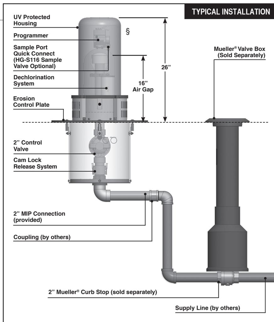
6. Disinfect the Hydro-Guard® Flushing Device in accordance with the utility's policy. DO NOT exceed the dosage and contact times recommended by the AWWA.
