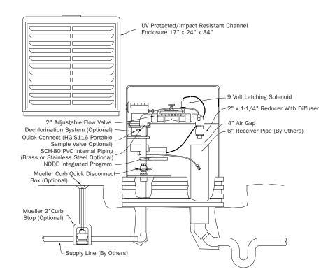
**5.** Backfill the hole around, under, and inside of the Unit with clean fill and/or #57 stone. Backfilling should be accomplished in 6" compacted lifts. Check that the Unit Is level. **6.** Disinfect the Hydro-Guard<sup>®</sup> Flushing Device in accordance with the utility's policy. DO NOT exceed the dosage and contact times recommended by the AWWA.
