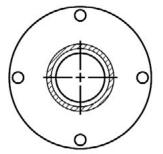
$\frac{3}{4}'' \phi$  (19 mm) Bolt Holes on 10  $\frac{1}{2}'' \phi$  (267 mm) Bolt Circle
