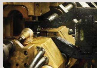
Stem is electrically heated and thrust collar is formed together to create the thrust collar
