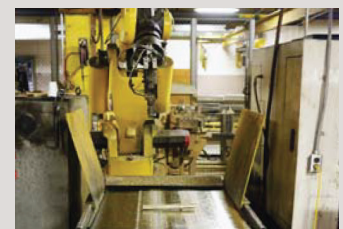
Stem threads and thrust collar are robotically machined and sorted
