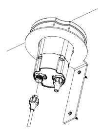
Plug sensor cable into RTU and rotate nut 1/4 turn counter-clockwise.
