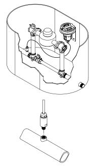
2 Apply joint-sealant and thread pressure sensor into 1/4" NPT port. Turn on the water.
