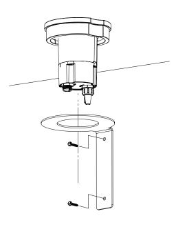
Install mounting bracket to wall of meter box/vault.
