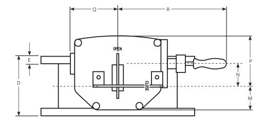
**Note:** Dimensions +/–  $\frac{1}{16}$ " (1.5 mm) up to 10"/DN250 valves, +/–  $\frac{1}{16}$ " (3 mm) for 12"/DN300 and larger valves.
