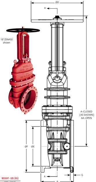
\*Resilient Wedge OS&Y Valves with similar performance and features, but different bonnet construction are available in 2″- 12″/DN50 - DN300 sizes, model R-2361+.
