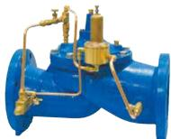
The M106-RPS and M206-RPS pressure sustaining valves control upstream pressure. Under flowing conditions, the pilot reacts to small changes in pressure to control the valve position. Should upstream pressure fall below the setpoint, the valve will close or modulate to ensure the setpoint is maintained.
