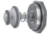
All parts of the Mueller Dual Check Valve are corrosion resistant for many years of dependable service. As of January 4, 2014, body and end-cap are made from low lead brass that complies with AWWA C800. Dual poppet assemblies are made of acetal plastic material with natural rubber gaskets, and springs are stainless steel.
