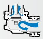
FULLY CLOSED Drain valves are open to allow drainage of barrel.
