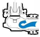
CLOSED The main valve held closed by operating nut & water pressure; barrel is dry.
