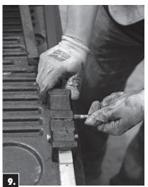
**9.** Remove existing clevis pin from coupling (coupling to remain assembled to the nickel plated top rod). Then remove rod guide currently on the lower rod.
