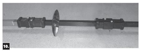
**10.** Assemble coupling (ID-4) to the lower rod. Slide the rod guide on to the newly installed extension rod 5-6" below the end of the rod. Then, reinstall the top rod.
