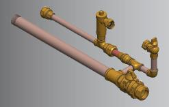
Developed for cities requiring residential fire sprinklers, this compact fitting is designed to support a <sup>3</sup>/<sub>4</sub>" meter and features two outlets: a lockable ball valve on the domestic side and unimpeded flow to the fire protection system on the other. Made from low-lead brass, it complies with NFPA 13D and avoids on-site assembly of multiple components.
