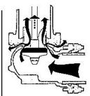
Closing—water pressure again force-flushes drain valves.
