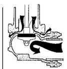
Closed—drain valves are open to allow complete drainage from barrel.
