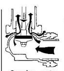
Opening—water pressure forceflushes double drain valves and drain openings.
