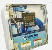
The LCP-TP Single Process Level Controller is designed to complement Singer's single solenoid operated/override control valves and sensor. it is programmed with customized level control algorithms and offers both local control via interactive display or remote control via 4-20mA or Serial Modbus SCADA communication. For more information, please visit www.singervalve.com.
