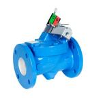
non-slam construction ensures dependable, maintenance-free performance, while its large, unobstructed flow path makes the valve an excellent choice for wastewater as well as water applications. Additionally, the mechanical joint end connection and 316 stainless steel cover bolt option is designed for buried installation that avoids the expense of vault construction. For more information, please visit <a href="https://www.prattvalve.com">www.prattvalve.com</a>.
