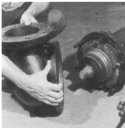
5. Position Shoe to slip in place.
