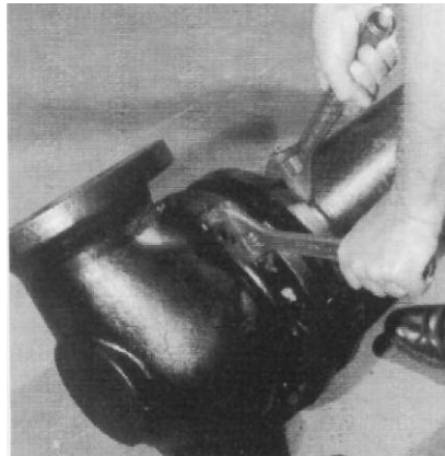
7. Replace Shoe Bolt Nuts. Tighten to approximately 1800 in-lbs.
